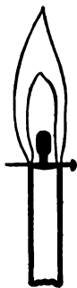
FIG. 10.—Match head in flame shows that combustion occurs at the surface only.
